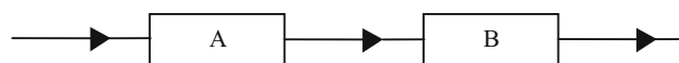
Fig. 1 “Series” combination of two components A and B , where the ability of B to do anything useful relies on the correct functioning of A . The combination only functions correctly if both A and B are functioning normally. The arrows indicate the sequence of any dependency, e.g. of data flow
