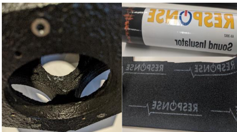
Figure 3.7 Dodecahedron enclosure lined with sound absorption material
