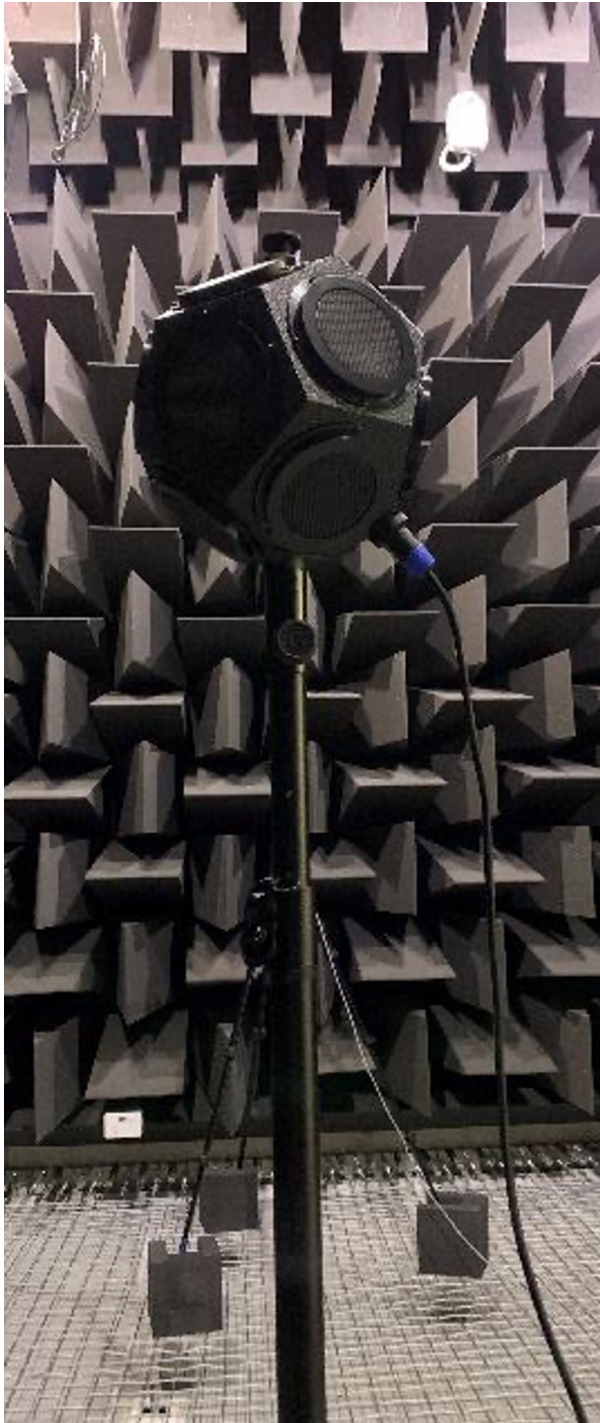
Figure 3.17 Final dodecahedron loudspeaker during testing in the UTS Tech Lab anechoic chamber
