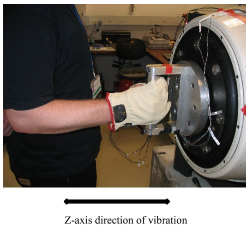
Fig. 4 A glove test set-up, testing in compression in the z -axis
