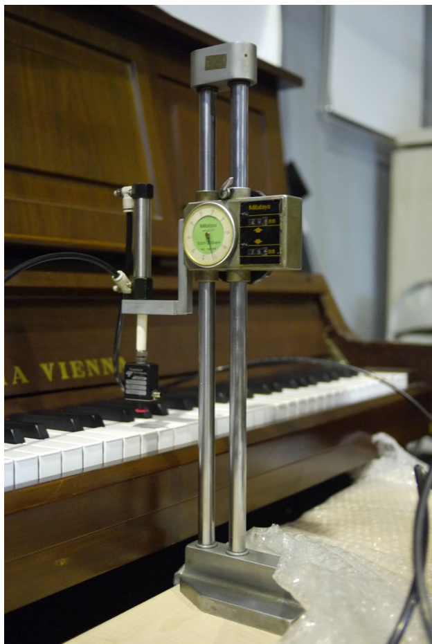
Fig. 2 Customized calibrated system with load cell of MDB-50
