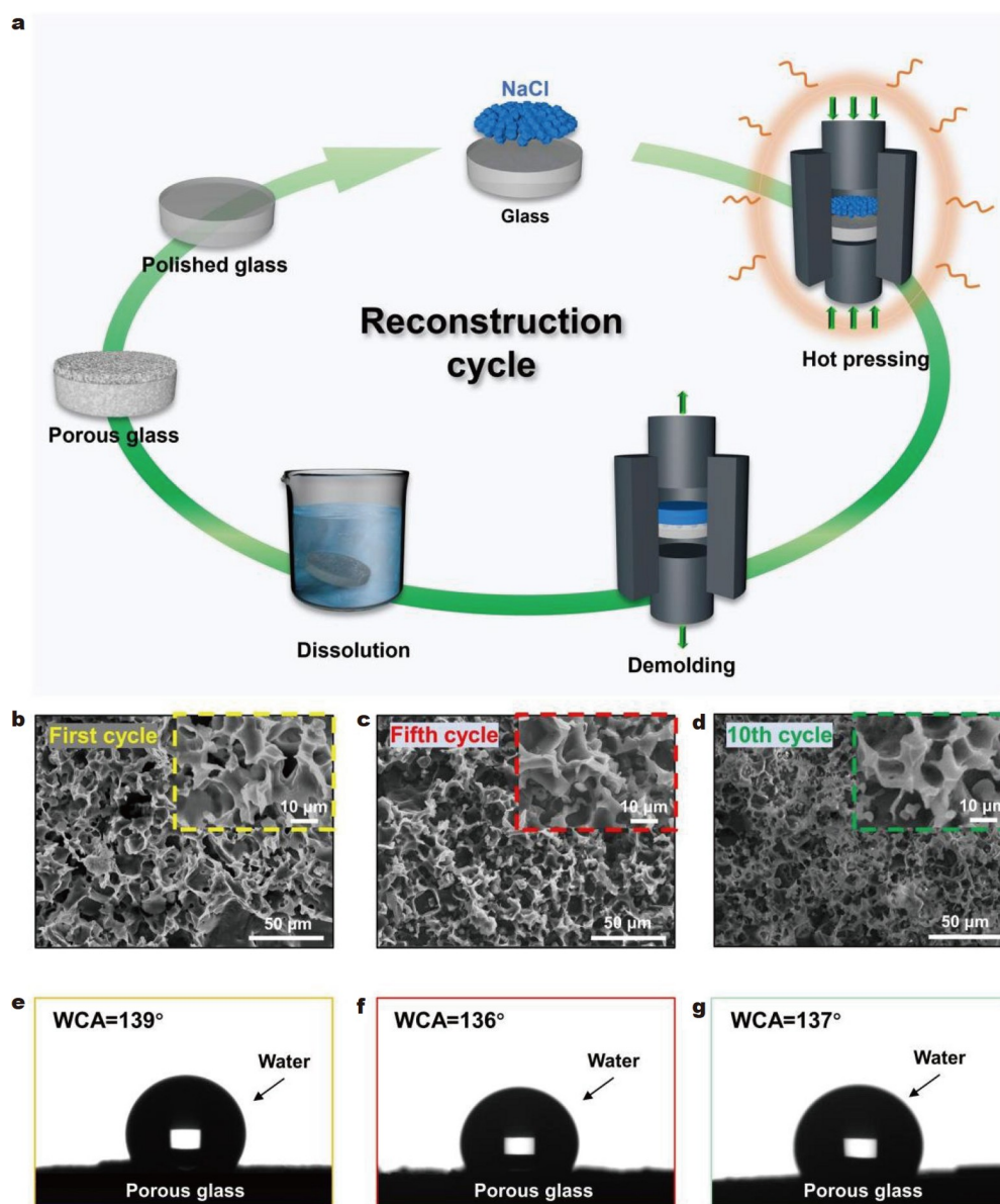
Figure 5 (a) Reconstruction of the porous glass. (b–d) SEM images of the porous glass fabricated in the first, fifth, and tenth cycles, respectively; (e–g) WCA values of the porous glass fabricated in the first, fifth, and tenth cycles, respectively.
