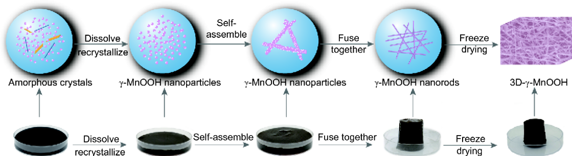
Figure 1 Schematic of the preparation of 3D- \gamma -MnOOH via hydrothermal reaction and freeze-drying.
