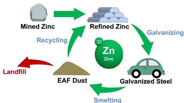
Fig. 1 Schematic of the mass flow of Zn in steel industry
