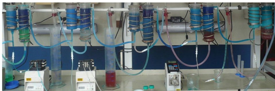
Fig. 4 Continuous extraction process for the separation of cobalt from nickel with the ionic liquid Cyphos IL 101 as the extraction phase. The different stages are (from left to right): an extraction stage, a washing stage and three stripping stages in counter-current mode.
