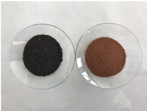
Fig. 3 Appearance of OS, before (left) and after (right) thermal treatment
