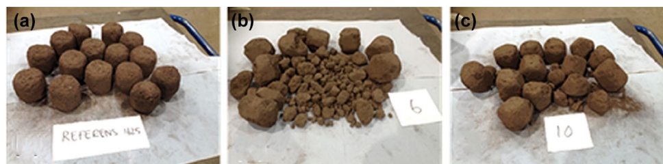
Fig. 1 Photograph of briquettes after tumbling: a FR0; b R6; c R10. FR0: standard briquette
