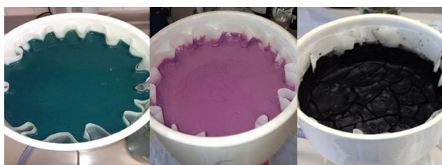
Fig. 4 Formation and filtration of Co, Ni and Mn precipitates (from left to right : metal hydroxide, metal carbonate and metal sulphide)
