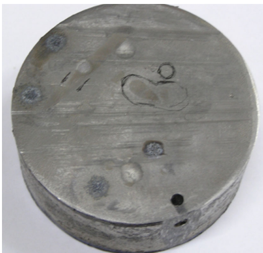
Fig. 2 Cross section of a medium size ingot after first remelting (target composition Ti–22Nb–6Ta)
