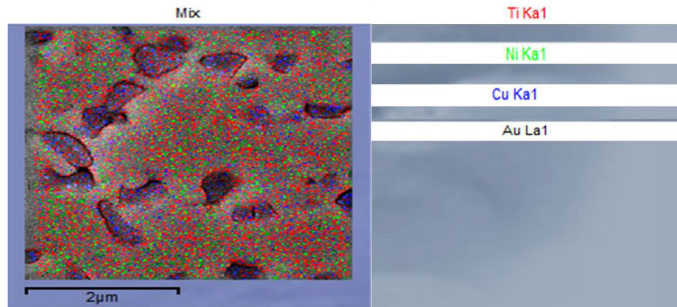
Fig. 6 X-ray mapping of 10Cu alloy annealed at 973 K showing distribution of alloying elements
