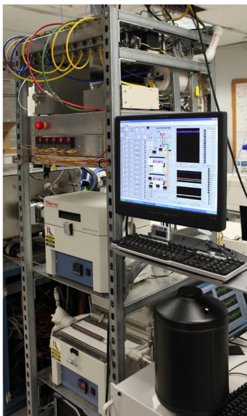
Fig. 2 Flow reactor with PF loaded in quartz reactor in bottom furnace
