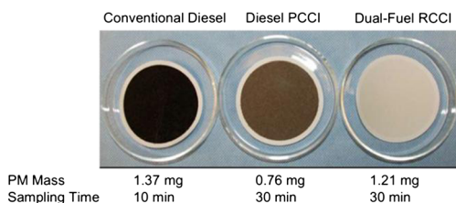
Fig. 3 Particle mass samples collected on Teflon-coated quartz-fiber filters for conventional diesel, diesel PCCI, and dual-fuel RCCI combustion at 2300 RPM, 4.2 bar BMEP [23]
