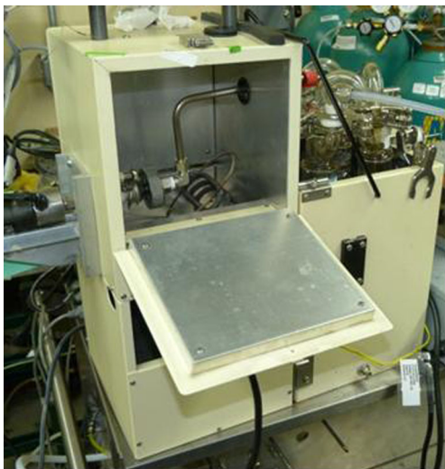
Fig. 6 Filter oven for sampling raw exhaust. The impinger glassware downstream of the filter is to condense water out prior to sample volume measurement with a dry gas meter
