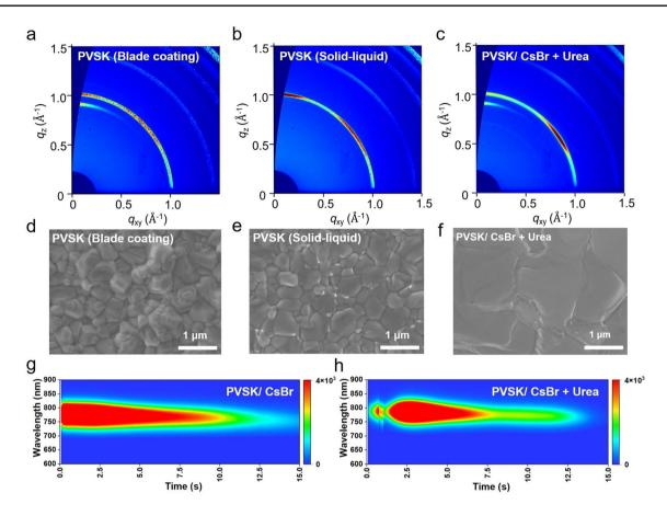
Fig. 3 a, b 2D GIWAXS patterns of pristine perovskite film (prepared by blade coating and solid–liquid deposition), and c the perovskite film modified with CsBr+Urea. Note that the modified perovskite films were prepared using a solid–liquid strategy. d-f SEM images of corresponding pristine and modified perovskite films. Heat maps of in situ PL for g PVSK/CsBr and h PVSK/CsBr+Urea
