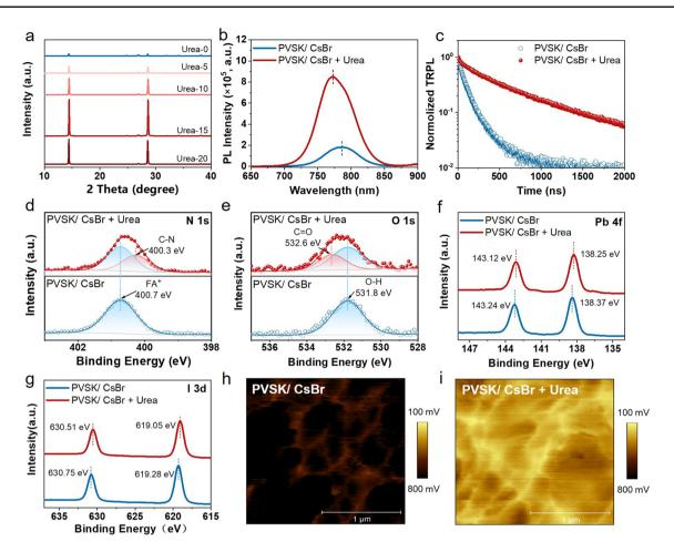
Fig. 4 a XRD patterns of perovskite films modified with buried CsBr and vary concentrate Urea. b PL and c TRPL spectra of the PVSK/CsBr and PVSK/CsBr+Urea films. XPS spectra of d N 1s, e O 1s, f Pb 4f, and g I 3d for PVSK/CsBr and PVSK/CsBr+Urea films. The KPFM images of h PVSK/CsBr and i PVSK/CsBr+Urea films
