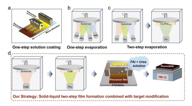
Fig. 1 Illustrations of common large-area perovskite deposition methods, including **a** solution-processing techniques (blade coating, slot die coating, and spray coating), **b** one-step thermal evaporation, and **c** two-step thermal evaporation techniques. **d** The strategy of the perovskite film preparation in this work: solid–liquid two-step film formation combined with target modification
