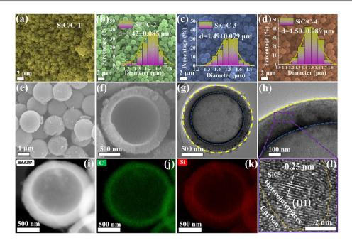
Fig. 2 Low-magnification SEM images of a SiC/C-1, b SiC/C-2, c SiC/C-3, and d SiC/C-4, and the insets are the corresponding statistical distribution of diameters. e-f High-magnification SEM images of SiC/C-3. g-h TEM images of SiC/C-3. I-k The corresponding element mapping images and I HR-TEM image of SiC/C-3
