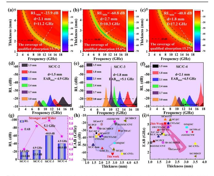
Fig. 4 2D RL mapping of a SiC/C-2, b SiC/C-3 and c SiC/C-4. RL curves below -10 dB at given absorber thickness of d SiC/C-2, e SiC/C-3 and f SiC/C-4. g The frequency dependence of  $RL_{min}$  and EAB values of all samples with the optimal thicknesses. h Comparison of  $RL_{min}$  values and i EABs among previously reported silicon carbide and carbon related MAMs
