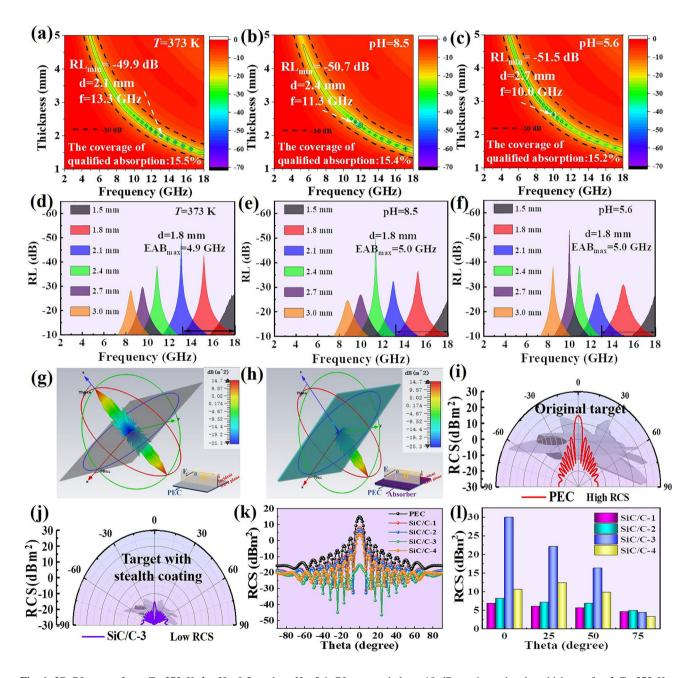
**Fig. 6** 2D RL maps for **a** T=373 K, **b** pH=8.5, and **c** pH=5.6. RL curves below -10 dB at given absorber thickness for **d** T=373 K, **e** pH=8.5, and **f** pH=5.6. **g** 3D radar wave scattering signals of PEC and **h** PEC coated with SiC/C-3. **i** RCS simulated curves and **k** RCS in polar coordinate system of PEC and **l** PEC plate coated with SiC/C-3 at 14.0 GHz. **j** RCS reduction values of PEC and PEC coated with different SiC/C composites
