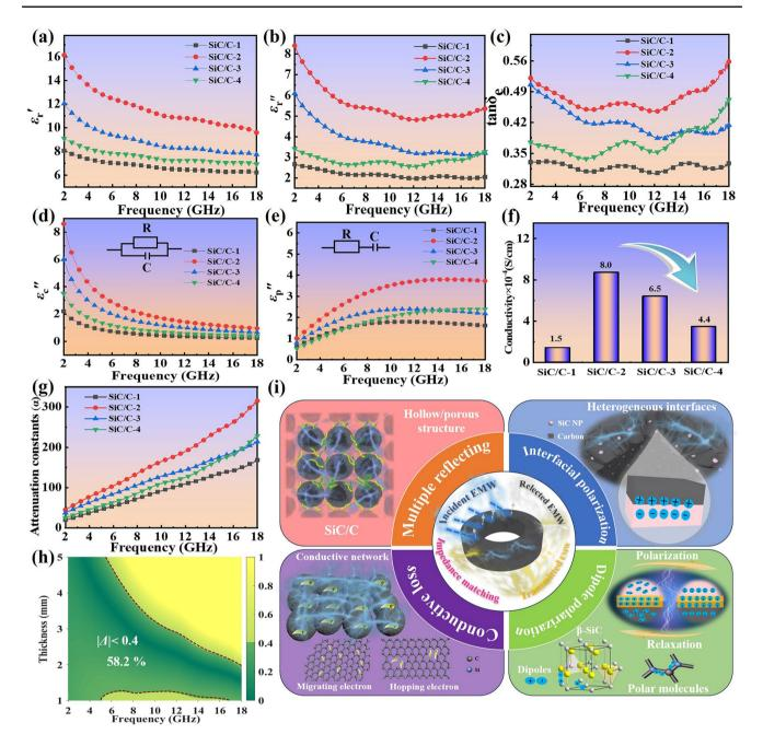
Fig. 5 Frequency-dependent **a**  $\varepsilon_r'$  curves, **b**  $\varepsilon_r''$  curves, **c** dielectric loss tangent (tan $\delta \varepsilon$ ), **d** fitted conductivity loss, **e** fitted polarization loss, **f** conductivity values, **g**  $\alpha$  curves of SiC/C composites. **h** 2D  $|\Delta|$  map and **i** schematic illustration for the microwave absorption mechanisms of SiC/C-3
