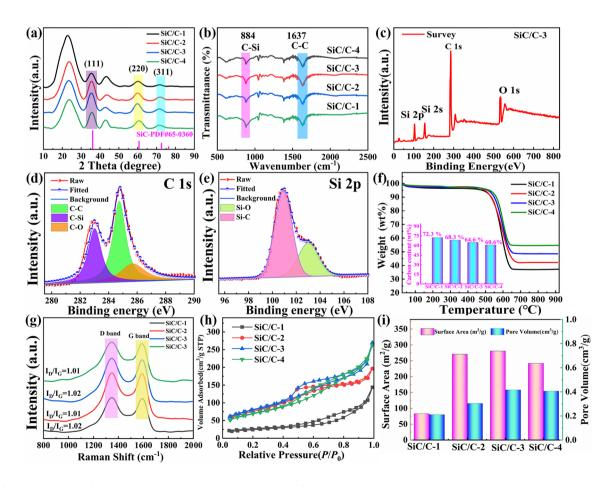
Fig. 3 a XRD patterns, b FT-IR spectra, c-e XPS survey spectra, and f TG curves (Inset is the calculated contents of carbon), g Raman spectra, h  $N_2$  adsorption–desorption isotherms, and i the histograms of BET surface areas and pore volumes of SiC/C composites
