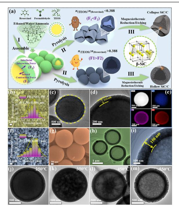
**Fig. 1** a Preparation mechanism diagram of SiC/C composites. **b** SEM images, **c-d** TEM images and **e** the corresponding element mapping images of PR@SiO<sub>2</sub>/PR-3. **f-g** SEM images and **h-i** TEM images of SiO<sub>2</sub>/C-3. **j-m** TEM images with different pyrolysis temperature (250, 350, 450, and 550 °C) of SiO<sub>2</sub>/C-3
