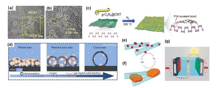
**Fig. 5 a**, **b** HRTEM images of  $Ni_3S_2$  quantum dots. Reprinted with permission from Ref. [100]. **c** Schematic illustration of 2D BP-CN-c. Reprinted with permission from Ref. [99]. **d** A diagrammatic representation of electrolyte diffusion state on hollow CoFe–NC–x. Reprinted with permission from Ref. [102]. **e**–**g** CoO and Ni–Fe-layered double hydroxide with CNT hybrids for the electrocatalysis of ORR and OER. Reprinted with permission from Ref. [47]
