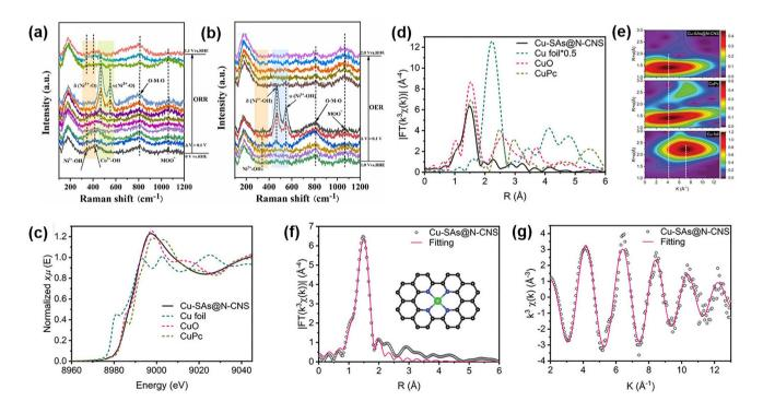
**Fig. 15** In situ Raman spectra collected on CoNi-CoN<sub>4</sub>-HPC-900 for **a** the ORR process and **b** the OER process in 0.1 M KOH solution. Reprinted with permission from Ref. [223]. **c** Cu K-edge XANES, **d** FT  $k^3$ -weighted Cu K-edge EXAFS, and **e** WT-EXAFS spectra of Cu-SAs@N-CNS and Reference samples. **f**, **g** FT-EXAFS fitting curves for Cu-SAs@N-CNS in R and K spaces. Reprinted with permission from Ref. [211]
