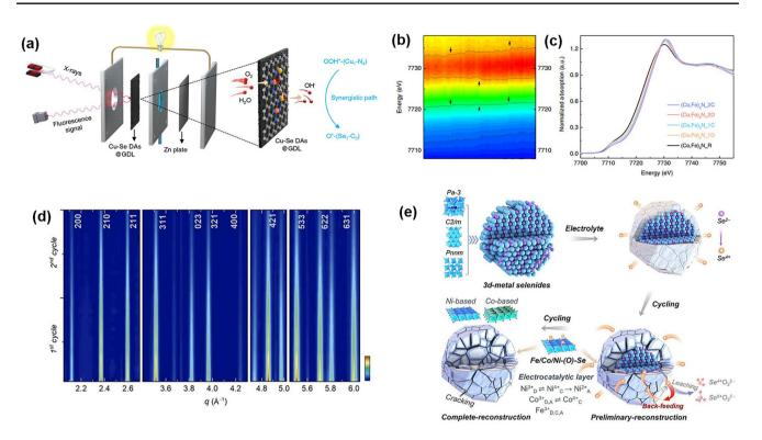
**Fig. 16** a Illustration of operando XAS set up for ZAB under realistic device working conditions. Reprinted with permission from Ref. [230]. **b**, **c** The operando XANES spectra of Co. Reprinted with permission from Ref. [192]. **d** Operando 2D HEXRD contour map of (Fe, Ni)Se<sub>2</sub> in a Zn–air battery. **e** Schematic demonstration of the Se-driven reconstruction mechanism. Reprinted with permission from Ref. [231]
