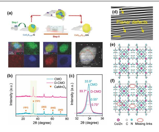
Fig. 9 a Schematic illustration of the synthesis of  $CoO_{0.87}S_{0.13}/GN$ . Reprinted with permission from Ref. [158]. b, c XRD patterns, d FFT image of D-CMO. Reprinted with permission from Ref. [159]. Schematic diagram of the e intact ZIFs and f linker-deficient ZIFs. Reprinted with permission from Ref. [160]
