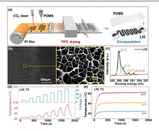
Fig. 2 Preparation and Joule thermal properties of the LIG TC. a Preparation process of the LIG TC. b SEM image of LIG (texture structure and porous structure). c XPS analysis of LIG. d Joule thermal properties LIG TC. e The heating stability of the LIG TC
