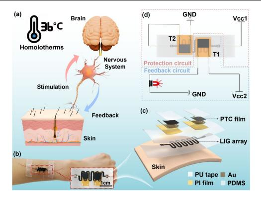
Fig. 1 Design concepts and system features of the interactive thermo-regulation bionic electronic system (TRES). a Temperature self-regulation mechanism in homoiotherms. b The actual picture of TRES placed on the arm. c Temperature self-regulation mechanism of TRES. d Assembly diagram of TRES
