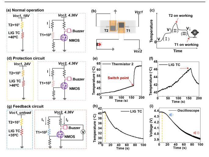
Fig. 4 Circuit design and self-regulating performance of TRES. a Circuit diagram in normal working condition. b Schematic diagram of connection mode of protection circuit and feedback circuit. c Working mechanism of different thermistors. d Protection circuit diagram. e Real-time temperature during T2 working. f The temperature change of LIG TC on T2 working. g Feedback circuit diagram. h The temperature change of LIG TC on T1 working. i The indicator of oscilloscope changes in real time
