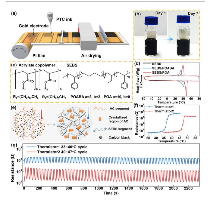
Fig. 3 Preparation and thermo-response properties of PTC thermistors. a Preparation process of PTC thermistors. b The stability of PTC ink. c Molecular formula of functional polymers. d Melting and crystallization capacity of acrylate copolymers. e Working mechanism of PTC thermistors. f Temperature response performance of PTC thermistors. g The response stability of PTC thermistors
