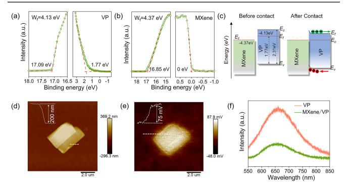
Fig. 2 UPS spectra of a VP and b MXene. c Band structure diagram of MXene and VP before and after forming heterojunction. d The AFM image of the MXene/VP heterojunction. e KPFM image corresponding to d. f PL spectra of the pure VP and MXene/VP hybrid film upon excitation at 532 nm
