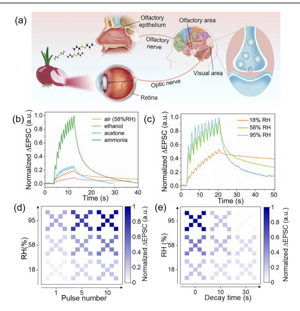
Fig. 6 a Schematic diagram of crossmodal interaction between vision and olfaction in the human perceptual system. b  $\Delta$ EPSCs triggered by 10 successive light pulses in environments with different gas atmospheres. c  $\Delta$ EPSCs triggered by 10 successive light pulses in environments with different RH. The d recognition and e forgetting process of the letter "X" pattern in environments with different RH
