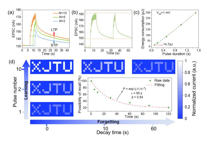
Fig. 5 a The transition from STP to LTP by increasing the number of light pulses. **b** The "learning-experience" behavior of the MXene/VP optoelectronic synapse. **c** The energy consumption of the MXene/VP optoelectronic synapse. **d** Normalized EPSC mapping images with a "XJTU" letter pattern under increasing light pulse numbers (vertical axis) and decay time (horizontal axis). The inset is the image forgetting process fitted with the Ebbinghaus forgetting curve
