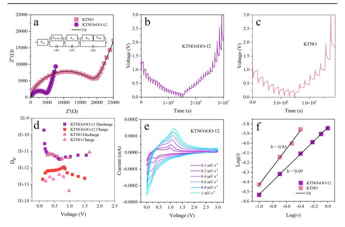
**Fig. 5** Electrochemical kinetics analysis of KTNO/rGO-12 and KTNO. **a** Nyquist plots of KTNO/rGO-12 and KTNO at OCP, with equivalent circuit as inset. **b** GITT potential profile of KTNO/rGO-12. **c** GITT potential profile of KTNO. **d** Corresponding  $D_K^+$  values **e** CV curves of KTNO/rGO-12 at scan rates from 0.1 to 1 mV s<sup>-1</sup>. **f** Relationship between the scan rate and the peak current of KTNO/rGO-12 and KTNO
