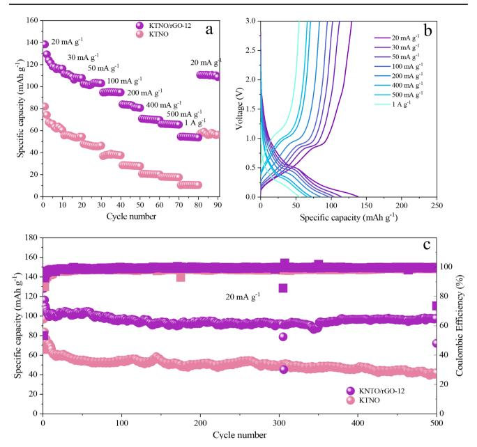
**Fig. 4** Rate and cycling performance of KTNO/rGO-12 and KTNO. **a** Rate performance comparison of KTNO and KTNO/rGO-12 between 20 mA  $\rm g^{-1}$  and 1 A  $\rm g^{-1}$ . **b** Galvanostatic charge–discharge curves of KTNO/rGO-12 between 20 mA  $\rm g^{-1}$  and 1 A  $\rm g^{-1}$ . **c** Long term cycling performance of KTNO and KTNO/rGO-12 at 20 mA  $\rm g^{-1}$  over 500 cycles
