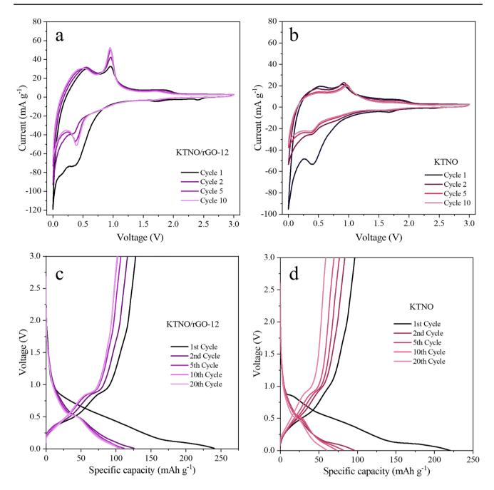
**Fig. 3** Electrochemical performance of KTNO/rGO-12 and KTNO. **a, b** CV curves of KTNO and KTNO/rGO-12 at 0.1 mV s<sup>-1</sup>. **c, d** Galvano-static charge–discharge curves of KTNO and KTNO/rGO-12 at 20 mA g<sup>-1</sup>
