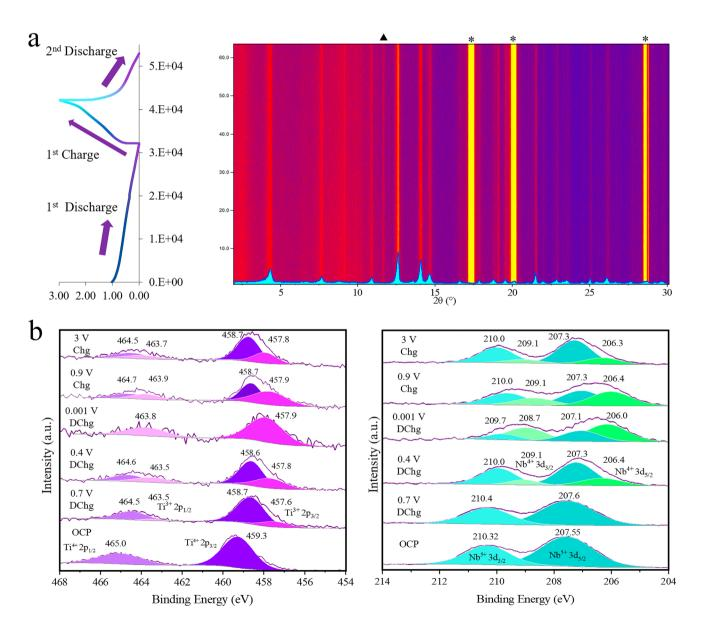
Fig. 7 Mechanistic analysis of charge storage. a In-situ XRD of KTNO/rGO-8 during the charge–discharge process with inset of pristine KTNO/rGO-8 XRD pattern (\*: Al; ▲: unidentified). b Ex-situ high resolution XPS spectra of Ti and Nb core lines at selected points along the charge–discharge curve
