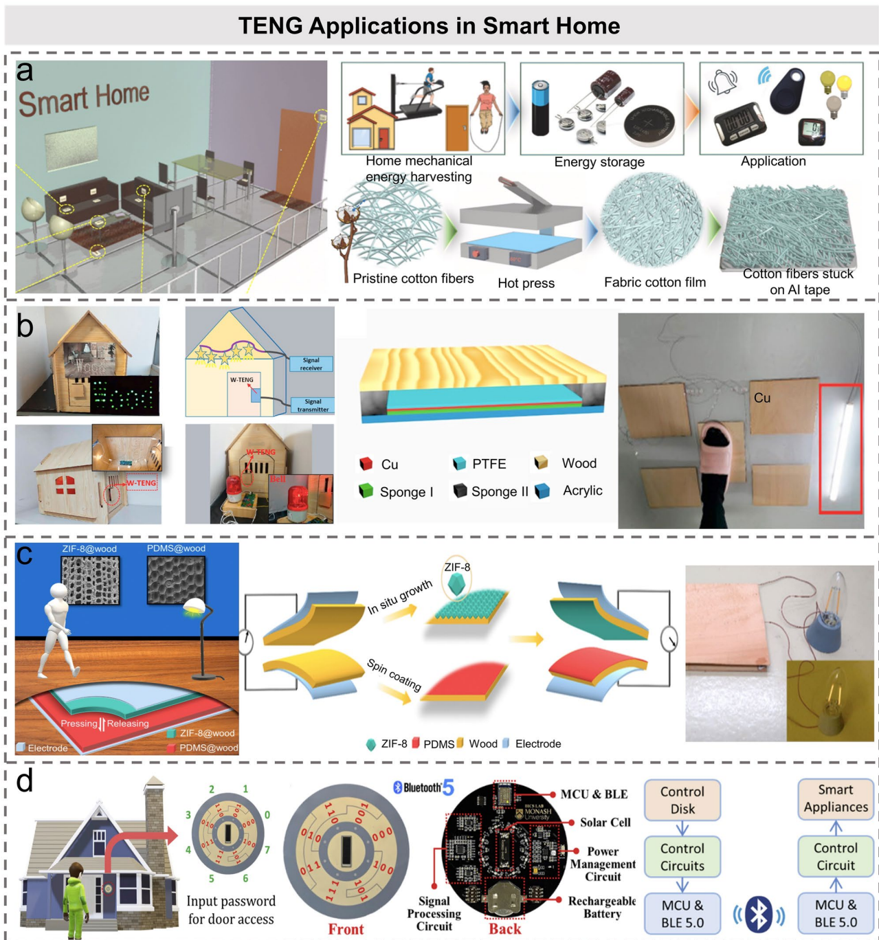
Fig. 7 TENG applications in smart home. a Schematic illustration of household mechanical energy, energy storage, and their applications [46]. Copyright 2020 Elsevier Ltd. b Application of W-TENG in smart home, and the schematic diagrams of W-TENG [110]. Copyright 2020 Elsevier Ltd. c Practical smart home applications of all wood-based TENG [147]. Copyright 2021 Elsevier Inc. d Illustration of the password authentication access control system. A password is required to enter the door and access control system [47]. Copyright 2020 Elsevier Ltd
