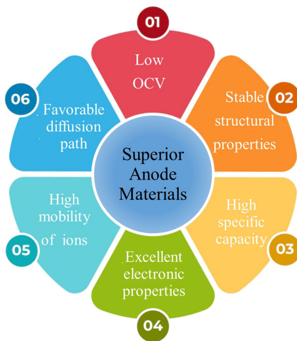
Fig. 17 Properties of a high-performing battery anode materials
