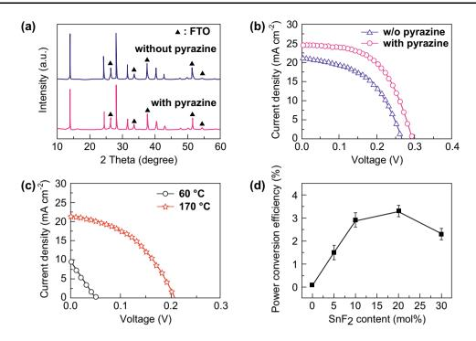
**Fig. 23** XRD patterns of FASnI<sub>3</sub> films **a** with and without pyrazine deposited on FTO glass, **b** with and without the presence of  $SnF_2$  (10 mol%), **c** in the absence of  $SnF_2$  annealed at 60 and 170 °C, and **d** PCE of the FASnI<sub>3</sub> and the amount of  $SnF_2$  added in the absence of pyrazine. Reproduced with permission Ref. [32]. Copyright ©2016 American Chemical Society
