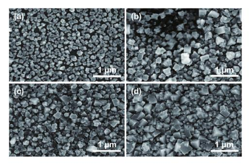
Fig. 21 SEM images of  $CH_3NH_3PbI_3$  films of different  $PbI_2$  concentrations: **a** 0.3 M, **b** 0.5 M, **c** 0.8 M, and **d** 1.1 M. Reproduced with permission Ref. [203]
