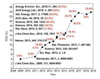
Fig. 4 Stepwise progress in perovskite solar cells demonstrating the remarkably sharp rise in photovoltaic performance over the past 8 years
