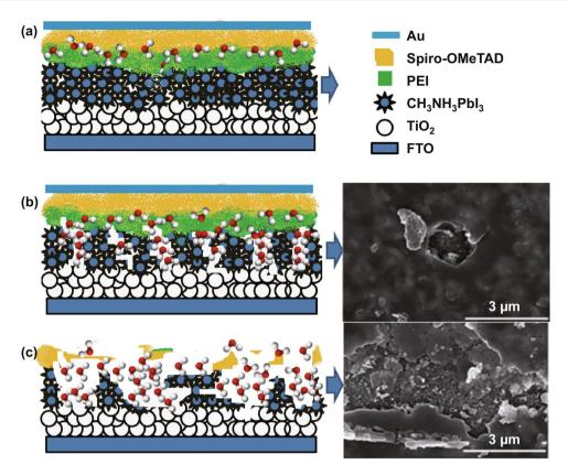
Fig. 19 Top view of the uncoated Au perovskite cell: a cell with PEI layer, b degradation of perovskite in the form of nanopinholes with PEI layer, and c degradation of cell randomly all over without PEI layer and corresponding SEM images. Reproduced with permission Ref. [196]. Copyright © 2015 The Royal Society of Chemistry
