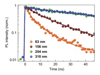
Fig. 20 Thickness-dependent time-resolved PL data illustrate PL decay curve of  $CH_3NH_3PbI_3$  films dipped at different concentrations of  $PbI_2$  upon excitation at 517 nm—the solid line corresponds to the results that are stretched exponentially. Reproduced with permission Ref. [203]
