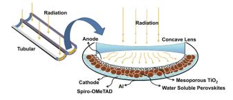
Fig. 26 Cross-sectional image of as-proposed low-cost model for water-soluble perovskite solar cells
