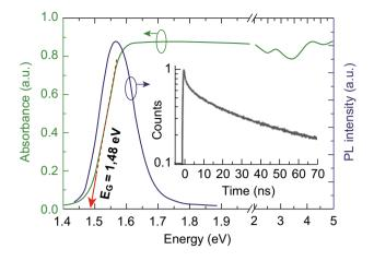
Fig. 13 UV-Vis absorption (green peak) and PL (blue) spectra of asground MAPbI3 measured at ambient temperature: fluorescence decay excitation measured at the 3.05 eV (inset view). Reproduced with permission Ref. [29]. Copyright © 2015 The Royal Society of Chemistry. (Color figure online)
