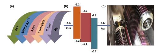
Fig. 17 Roll-to-roll fabrication of perovskite photovoltaic sheets
