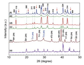
Fig. 14 XRD patterns of (a) CH<sub>3</sub>NH<sub>3</sub>I, (b) PbI<sub>2</sub>, (c) ball milling for 10 min, (d) ball milling for 45 min, (e) CH<sub>3</sub>NH<sub>3</sub>PbI<sub>3</sub>/Al<sub>2</sub>O<sub>3</sub>, and (f) CH<sub>3</sub>NH<sub>3</sub>PbI<sub>3</sub> by solution crystallization process. Reproduced with permission Ref. [135]. Copyright © 2016 Springer Science Business Media New York
