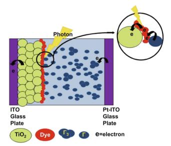
Fig. 3 Working principle of dye-sensitized solar cells
