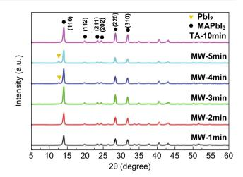
**Fig. 9** XRD pattern of perovskite films treated by 160-W microwave irradiation for 1, 2, 3, 4, and 5 min and annealed at 100 °C for 10 min. Reproduced with permission Ref. [27]. Copyright ©2016 American Chemical Society
