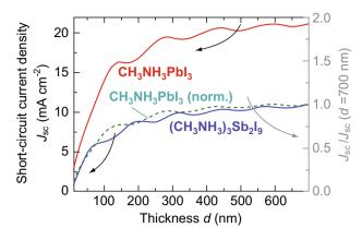
**Fig. 25** Plot of the thickness-dependent short-circuit current density  $J_{sc}$  of different perovskites. Reproduced with permission Ref. [236]. Copyright ©2016 American Chemical Society
