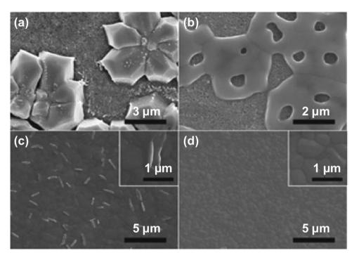
**Fig. 22** SEM images of FASnI<sub>3</sub> perovskite film fabricated using *N*,*N*-dimethylformamide (DMF) solvent **a** without nonsolvent dripping and **b** with nonsolvent dripping; SEM images of FASnI<sub>3</sub> perovskite film fabricated using mixed solvent of DMF and dimethyl sulfoxide (DMSO) with nonsolvent dripping, **c** the absence of pyrazine and **d** the presence of pyrazine. Reproduced with permission Ref. [32]. Copyright ©2016 American Chemical Society
