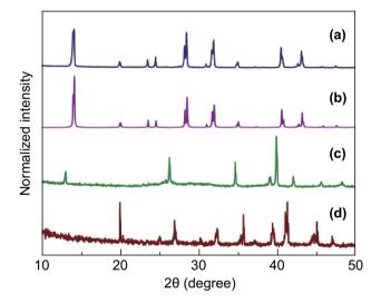
Fig. 12 XRD patterns of as-prepared material: (a) simulated MAPbI<sub>3</sub>, (b) as-ground MAPbI<sub>3</sub>, (c) PbI<sub>2</sub>, (d) MAI. Reproduced with permission Ref. [29]. Copyright © 2015 The Royal Society of Chemistry
