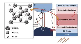
Fig. 1 a Simulated crystal structure of  $CH_3NH_3BX_3$  obtained from the diffraction pattern and **b** electron–hole diffusion diagram in the material
