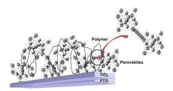
Fig. 16 Schematic view of the CH<sub>3</sub>NH<sub>3</sub>PbI<sub>3</sub> with ethyl cellulose
