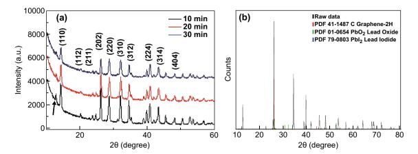
**Fig. 6** XRD patterns of  $CH_3NH_3PbI_3$  perovskite ultrafine nanoparticles: **a** after sonication in isopropanol for 10, 20, and 30 min (the peak assigned to unreacted PbI<sub>3</sub> is marked) and **b** after 20-min sonication in water. Reproduced with permission Ref. [109]. Copyright © 2016 Elsevier B.V.
