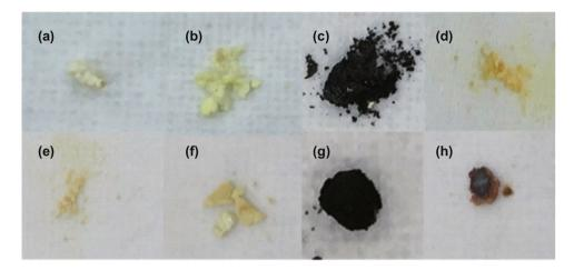
**Fig. 10** As-prepared perovskite material powder treated by microwave irradiation for **a** 0 min, **b** 1 min, **c** 2 min at 800 W and the  $PbI_2-CH_3NH_3I$  adduct powders treated by microwave irradiation for **d** 0 min and **e** 2 min and the  $PbI_2-CH_3NH_3I$  powders added with **f** diethyl ether, **g** DMF, and **h** DMSO treated by microwave irradiation for 2 min at 800 W. Reproduced with permission Ref. [27]. Copyright ©2016 American Chemical Society
