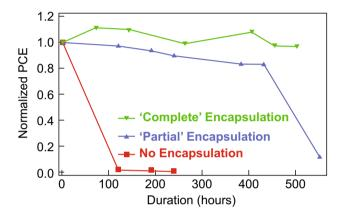
Fig. 18 Normalized I-V parameter of nonencapsulation, partial encapsulation, and complete encapsulation perovskites. Reproduced with permission Ref. [195]. Copyright © 2015 Elsevier Ltd.
