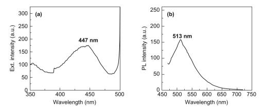
Fig. 8 a Excitation spectrum and b emission spectrum of CH<sub>3</sub>NH<sub>3</sub>PbI<sub>3</sub> nanoparticles. Reproduced with permission Ref. [109]. Copyright © 2016 Elsevier B.V.
