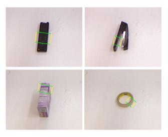
Fig. 1 Some example grasps for common objects, which are presented as oriented rectangles in 2D. Yellow lines represent the parallel plates of gripper, while green lines represent the opening width of the gripper before grasping
