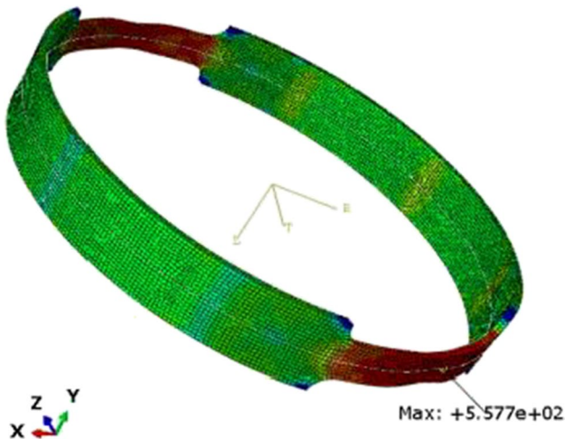
Fig. 11 The FEA ring specimen with an indication for the node having the maximum hoop stress value
