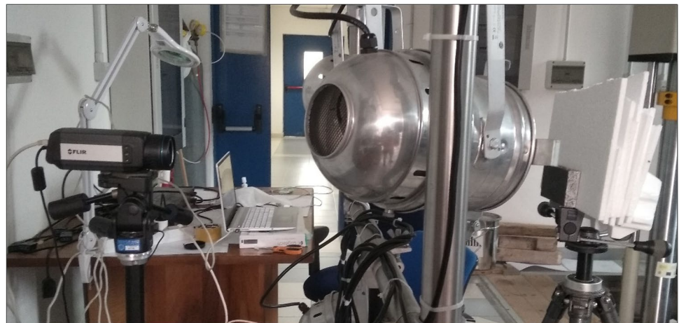
Fig. 6 Experimental pulsed thermographic setup for inspection of AFS elements
