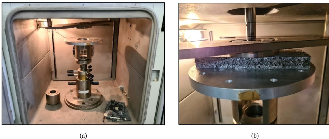
Fig. 3 (a) Clamping system and (b) AFS sample fixed with a rigid metallic circular plate (diameter equal to 40 mm)
