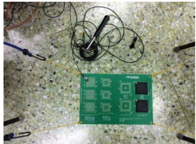
Fig. 8 Modal test setup in stage 2
