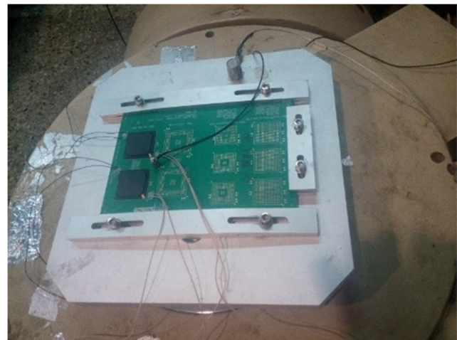
Fig. 17 Random vibration test set-up
