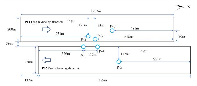
Fig. 5 GNSS monitoring stations location
