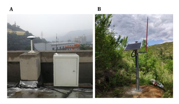
Fig. 6 Data acquisition base station and monitoring station. a GNSS base station b GNSS monitoring station
