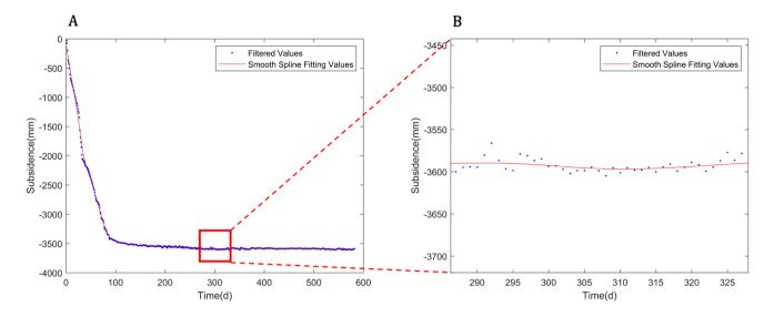
Fig. 9 Smooth processing of GNSS observation subsidence data. a Comparison before and after smoothing b The details of the comparison before and after smoothing
