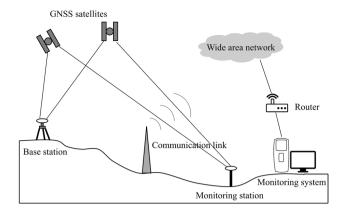
Fig. 2 Principle of GNSS online monitoring
