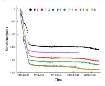
Fig. 7 The original observation subsidence data sequence of GNSS monitoring stations during the experiment
