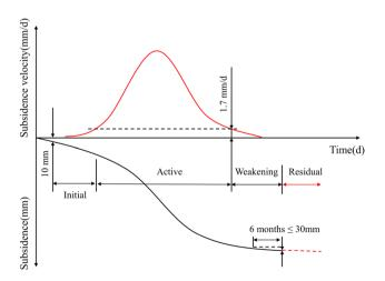
Fig. 1 Ground point subsidence development and subsidence velocity curve
