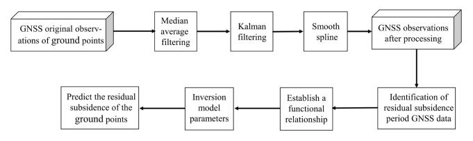
Fig. 3 Establishment process of residual subsidence model of arbitrary point on the ground of underground mining in mountainous areas based on GNSS online observation
