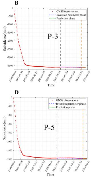
**Fig. 10** The comparison between the predicted value of the GNSS monitoring station based on the model in this paper and the measured value in the inversion parameter phase and the dynamic prediction phase. The black dotted line indicates the beginning period of resid-
