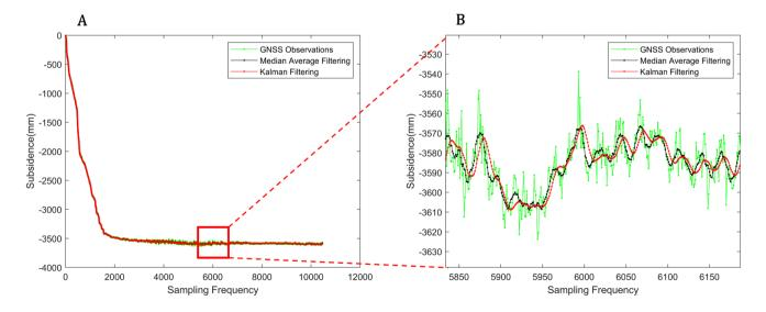
Fig. 8 Filter denoising processing of GNSS original observation subsidence data. a Comparison before and after filtering b The details of comparison before and after filtering
