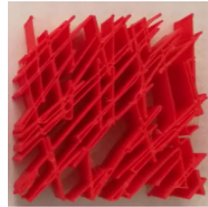
(b) 3D printed DFN model
