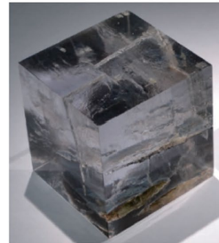
(c) 3D printed model of fractured coal and rock
