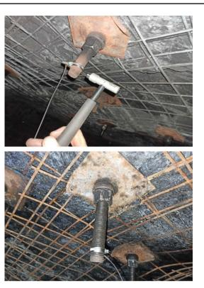
Fig. 2 An example of the test using impact hammer
