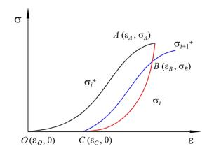
Fig. 1 Stress path of cyclic loading-unloading
