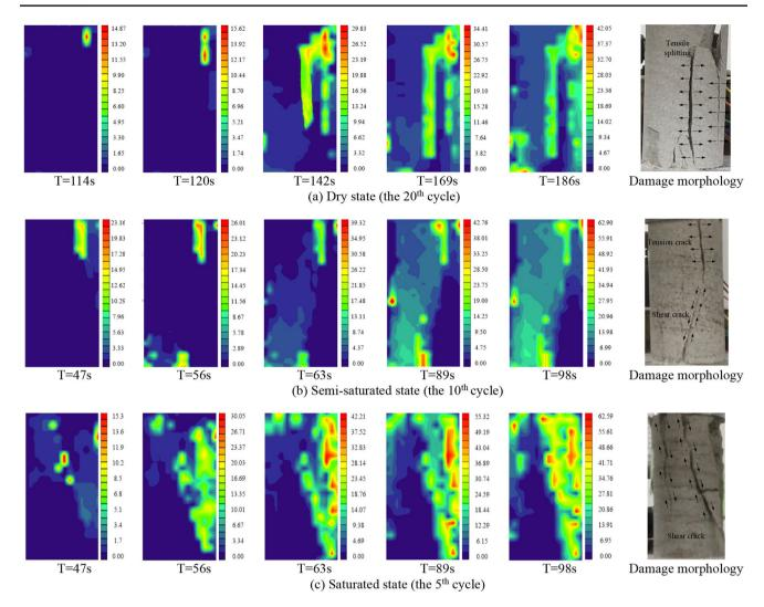
Fig. 14 Cloud maps of sandstone strain field with different water contents under graded cyclic loading-unloading conditions
