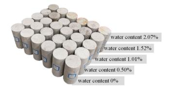
Fig. 3 Sandstone samples with different water contents
