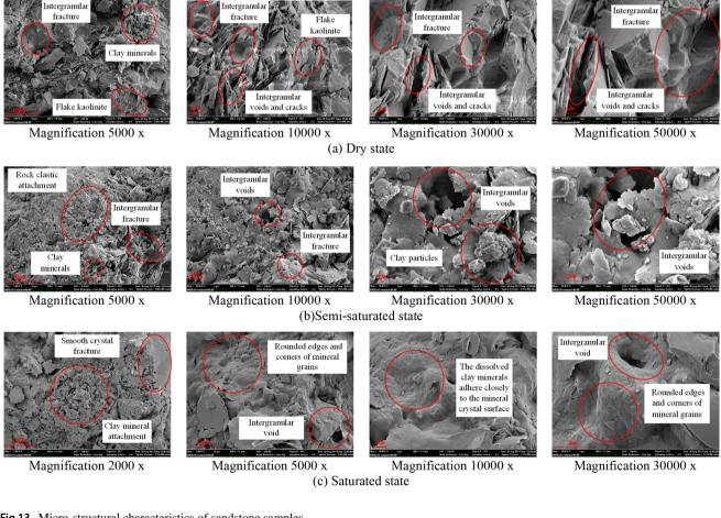
Fig.13 Micro-structural characteristics of sandstone samples
