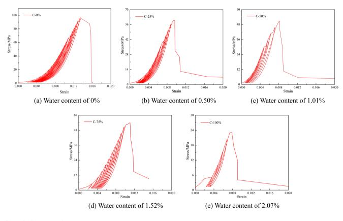
Fig. 8 Cyclic stress-strain curves
