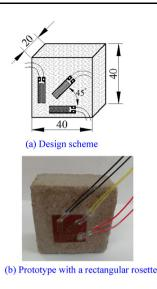
Fig. 10 Schematic and prototype of the strain brick
