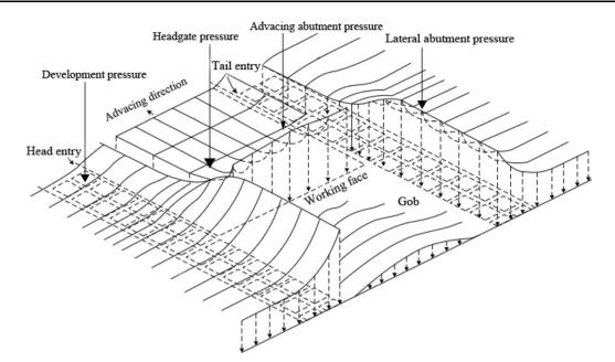
Fig. 1 Schematic of redistribution of vertical stress in a longwall panel (Peng 2019)
