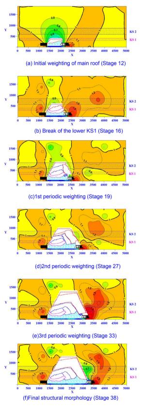
Fig. 14 Evolution of mining-induced vertical stress field
