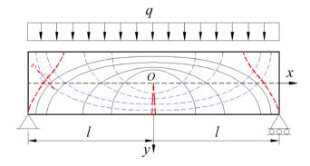
Fig. 15 Trajectories of principal stress before the initial breaking of the stratum
