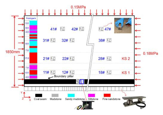
Fig. 4 Testing scheme of mining-induced stress field
