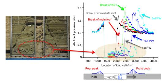
Fig. 12 Evolution of abutment pressure in different stages
