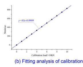
Fig. 7 Loading responses of the load cell
