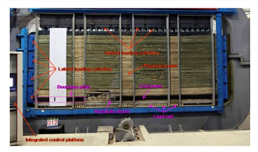
Fig. 3 Physical modeling system and application scenario
