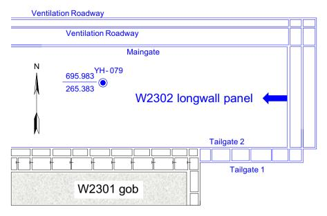
Fig. 2 The layout of W2302 longwall panel
