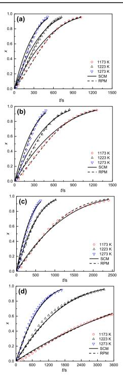
Fig. 5 Comparison of RPM-and SCM-predicted conversions to experimental values: a Py1073 char; b Py1173 char; c Py1273 char; and d MW char
