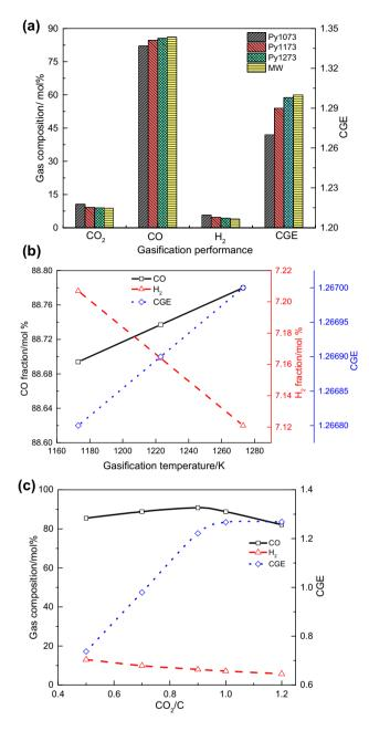
Fig. 7 Gasification performance of the char-CO<sub>2</sub> system: Effects of **a** the pyrolysis temperature, **b** the gasification temperature, and **c** the CO<sub>2</sub>/C molar ratio
