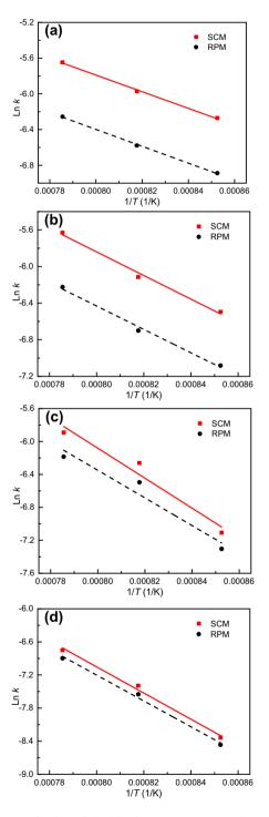
Fig. 4 Determination of the kinetic parameters (A and  $E_a$ ) from the SCM and RPM models: **a** Py1073 char; **b** Py1173 char; **c** Py1273 char; and **d** MW char
