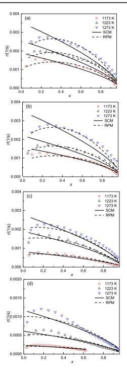
Fig. 6 Comparison of SCM- and RPM-predicted reaction rates to experimental values: a Py1073; b Py1173; c Py1273; and d MW char
