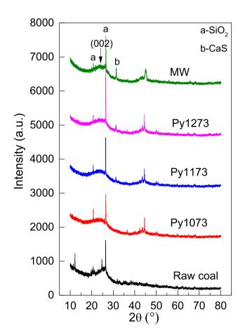
Fig. 1 XRD patterns from raw coal and pyrolyzed chars after conventional and microwave processing
