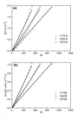
Fig. 3 Rate constant determination for the Py1073 char sample:  $a \; k_{\rm SCM}$  and  $b \; k_{\rm RPM}$
