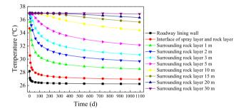
Fig. 5 Temperature distribution of roadway surrounding rock of basic working condition
