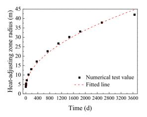
Fig. 4 Change and fitting of heat-adjusting zone radius of basic working condition
