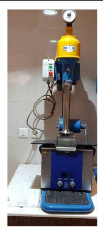
Fig. 2 The set up system for flotation
