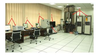
Fig. 1 MTS815 Rock Test System, which comprises six subsystems: 1—an acoustic three-dimensional positioning and collection system; 2—an MTS815 process control and acquisition system; 3—an ultrasonic excitation and acquisition system; 4—an MTS815 control center; 5—a high-temperature control system; 6—a loading system (axial, seepage, and confining pressures)
