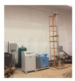
Fig. 4 The CBM well extraction simulator
