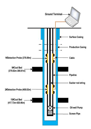
Fig. 7 Detection probe installation position
