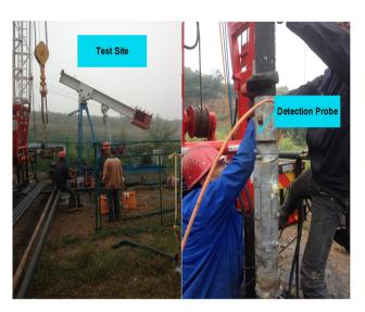
Fig. 8 Field photographs to show the detection probe entering a well
