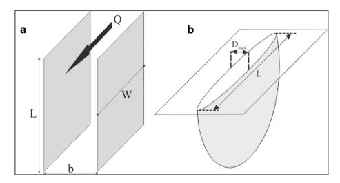
**Fig. 2** a Schematic diagram (modified after Klimczak et al. 2010) of fluid flow (*Q*) through parallel plates with length *L*, breadth *W*, and constant aperture width *b*. '*b*' is equivalent to  $D_{avg}$ . **b** Schematic diagram of an ideal isolated fracture with an elliptical opening profile having Length *L* and maximum aperture width  $D_{max}$
