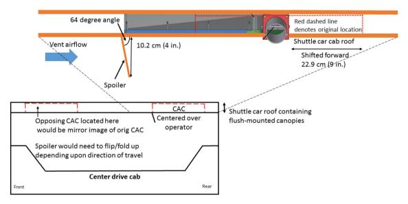
Fig. 11 Canopy air curtain built into cab roof, displaying forward shift of canopy location (9 in. forward) and spoiler to redirect ventilation airflow
