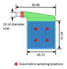
Fig. 5 The canopy air curtain showing gravimetric filter locations (measurements on figure are in centimeters)
