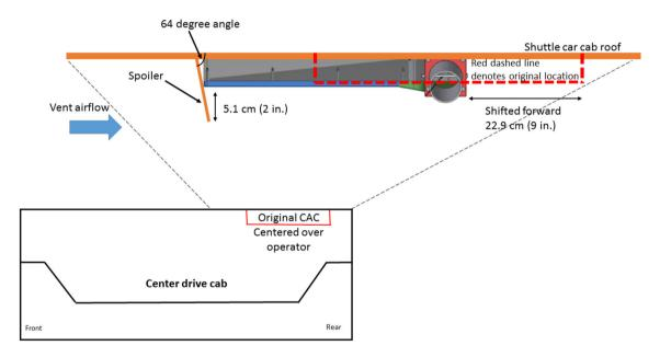
Fig. 9 Canopy air curtain underneath cab roof, displaying forward shift of canopy location 22.9 cm (9 in.) and spoiler to redirect ventilation airflow
