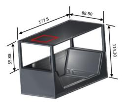
**Fig. 1** The center-drive shuttle car cab for the Joy 10SC32AA (dimensions in centimeters). The red outline shows the location of the canopy air curtain underneath the cab roof during testing (drawing by NIOSH)
