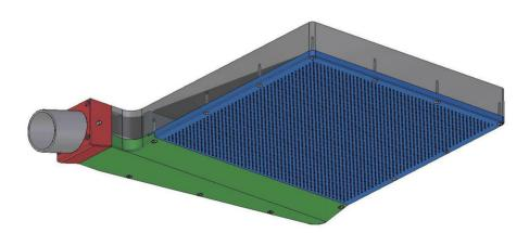
Fig. 3 The canopy air curtain underneath the roof of the shuttle car (drawing by Marshall University and J.H. Fletcher, Inc.)
