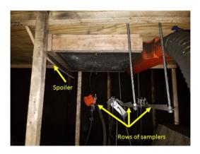
Fig. 10 Photo showing additional sampling row added to provide full sampling coverage underneath the CAC. Spoiler is shown on the front of the CAC
