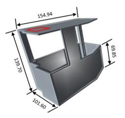
**Fig. 2** The end-drive shuttle car cab for the Joy 10SC32AB (dimensions in centimeters). The red outline shows the location of the canopy air curtain underneath the cab roof during testing (drawing by NIOSH)
