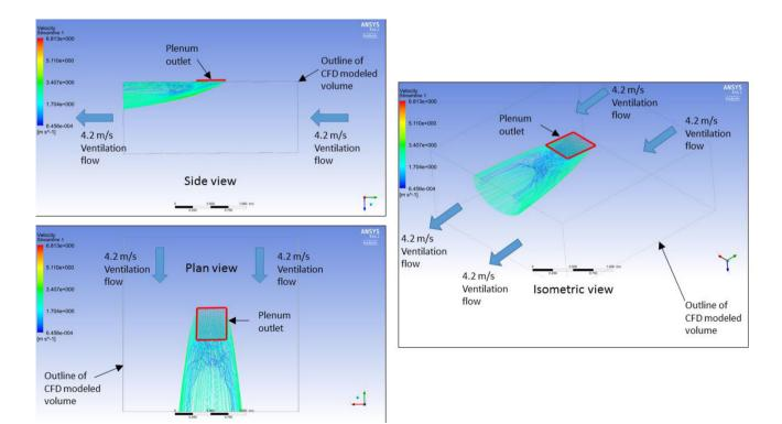
Fig. 7 CFD simulation results showing airflow streams from shuttle car CAC plenum in 4.2 m/s ventilation airflow (Marshall University)
