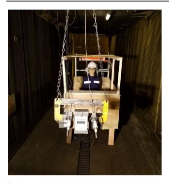
Fig. 4 Photo showing the setup of the center-drive cab for testing with the manikin used for centering the CAC over the shuttle car operator
