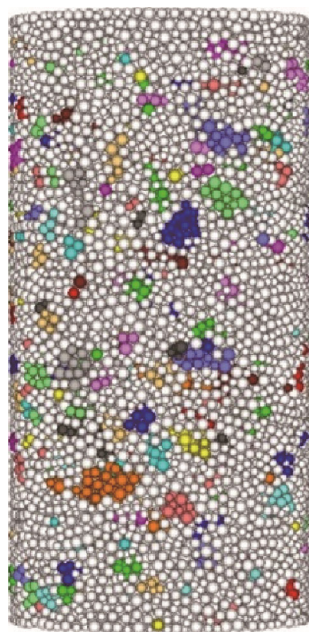
Fig. 8 A complete PFC3D model of SRM with a 30% rock ratio. The white color represents soil particles, and the other colors represent rock particles
