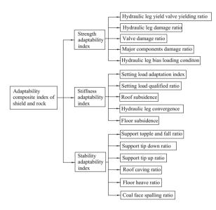
Fig. 3 Hydraulic support and surrounding rock adaptability evaluation indexes
