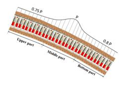
Fig. 10 Mining ground pressure distribution characteristics in steep dipping face  $% \left( \frac{1}{2} \right) = 0$
