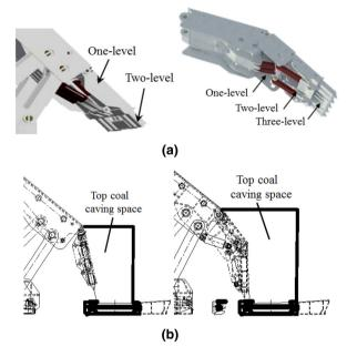
Fig. 7 Two types of top coal caving.  ${\bf a}$  Top coal caving device contrast,  ${\bf b}$  Top coal caving space contrast
