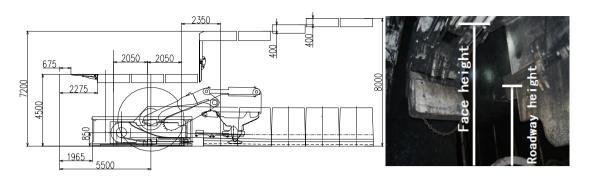
Fig. 5 Equipment matching manner for super cutting height working face
