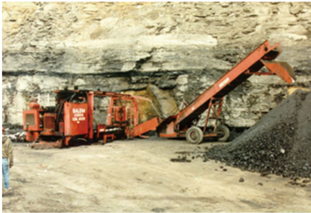
Fig. 6 Auger mining system in Indonesia
