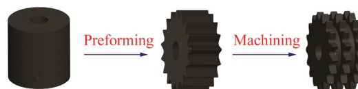
Fig. 2 Order of processing a multi-row sprocket
