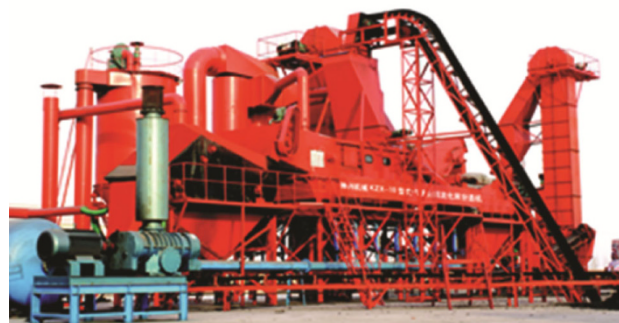
Fig. 2 Modularized industrial-scale ADMFB separator
