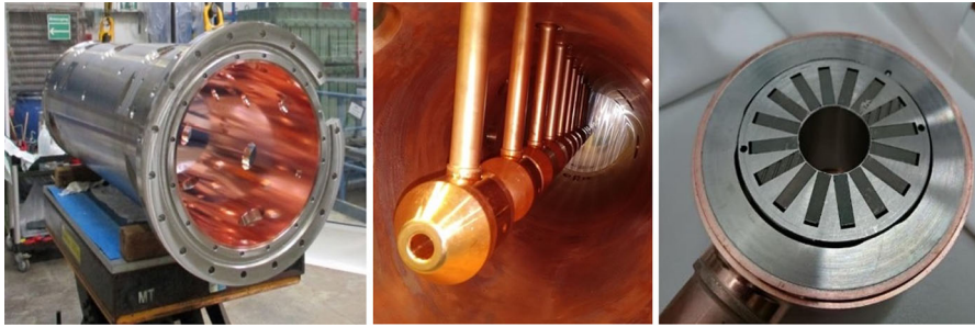
Fig. 9 Tank, drift tubes, permanent magnets during the assembly phase
