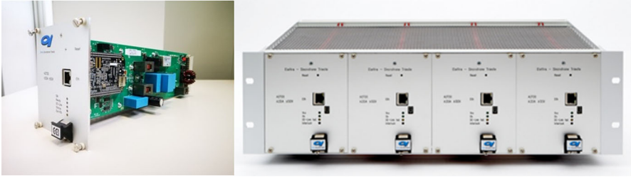
Fig. 19 One A2720 power converter and a 3U crate hosting four A2720 units
