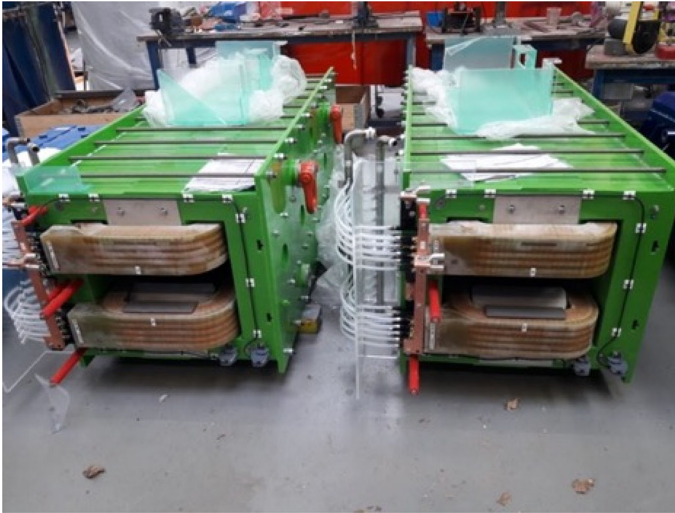
Fig. 17 The two dipole magnets
