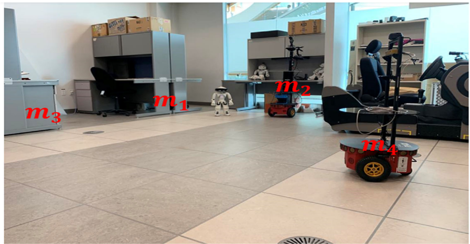
Fig. 2 Nao robot with HoloLens in indoor environment performing SLAM
