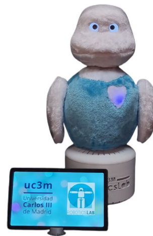
Fig. 2 The Mini social robot, the platform used to integrate the DMS, is dedicated to alleviating seniors' cognitive impairment by executing a broad repertoire of activities
