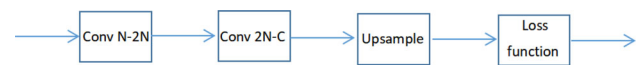
Fig. 2 The architecture of auxiliary feature extraction layer, N represents the number of channels, C represents the number of classes
