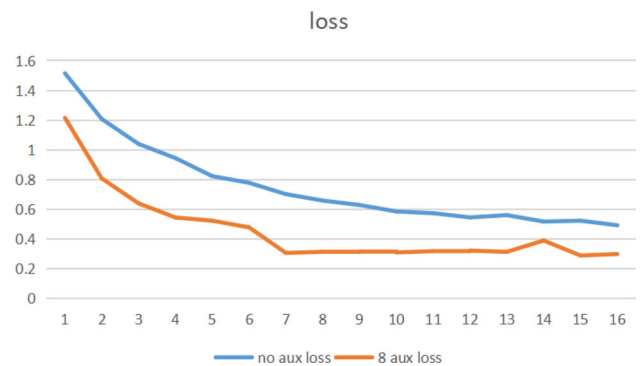
Fig. 3 Comparison of loss downward trend between using auxiliary feature extraction module and not using auxiliary feature extraction module
