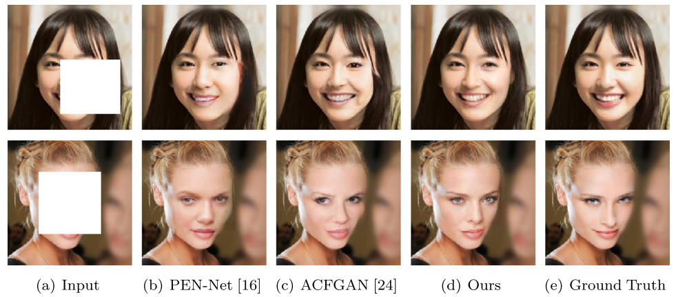
Fig. 9 Completing results on the CelebA-HQ dataset with random regular holes of a size between 64 * 64 and 128 * 128
